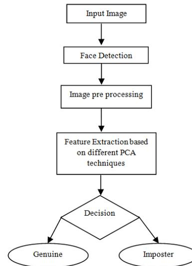
Figure 1. Face recognition system using Different PCA techniques
